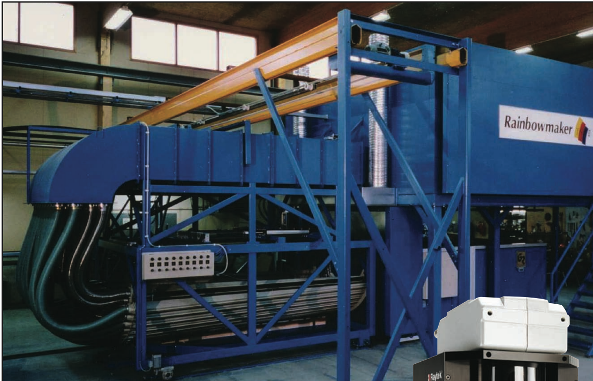
The GS150 provides real time temperature analysis for glass bending processes (Photo: Courtesy of Glassrobots OY, Tampere, Finland)
